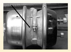
3. Insert the detachable release bolt through hole in head. Turn the release bolt clockwise until it stops and locks, then pull the release bolt out as far as possible, and run the nut down, holding the bolt in place.
